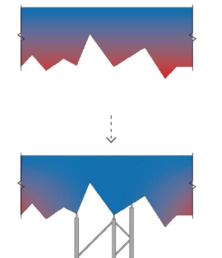
The lowest point of the structure has to be supported. Otherwise, the structure will fall down during printing.
