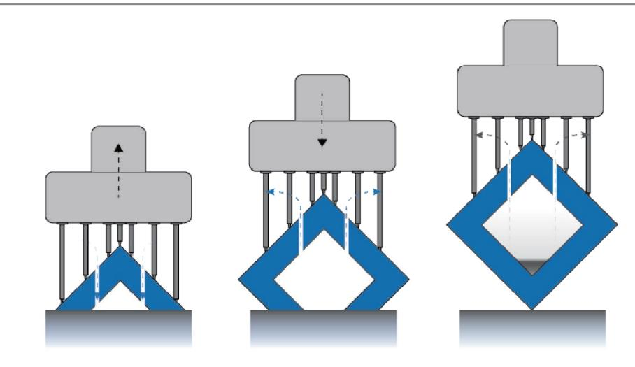
When the platform goes up, its inner air pressure will be reduced. In this way, the suction will grown so large that make it difficult to demold. Please lean the model to one direction in some degree to reduce the section as well as less supports will be needed. Add a hole on the bottom of the model to make sure liquid can be poured out and the stable air pressure.
