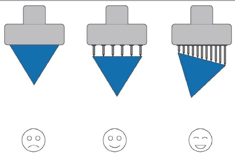
Models with flat bottom would be better to be printed after adding supports and base. It will be easier to take the model from platform and increase success rate greatly for models with base and supports Place the model at an appropriate angle to improve the success rate. Please note to add the supports evenly as well.
