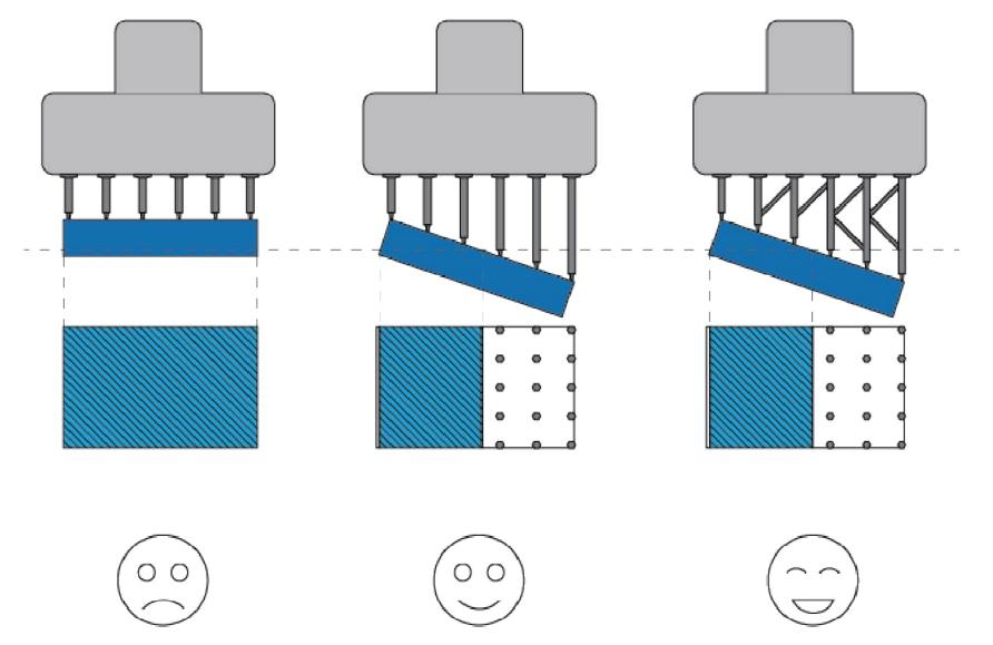
Models with big section is not suitable for printing, which probably damage the vat.
