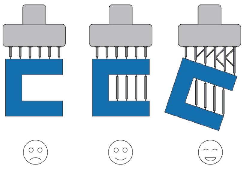
It is likely to lead to deformation in case of suspended structure without supports. Since the area of the model base is large, its section will be corresponding big and as we said above models with big section is not good for printing. Please lean the model to one direction in some degree to decrease the section. Meanwhile, less supports will be needed.
