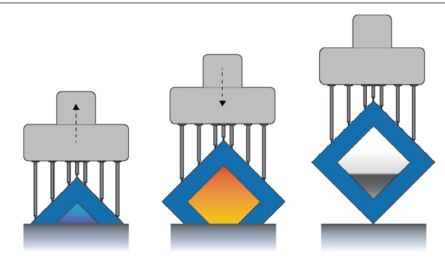
When the platform goes up, its inner air pressure will be reduced. In this way, the suction will grown so large that make it difficult to demold. Please lean the model to one direction in some degree to reduce the section as well as less supports will be needed. Add a hole on the bottom of the model to make sure liquid can be poured out and the stable air pressure.
