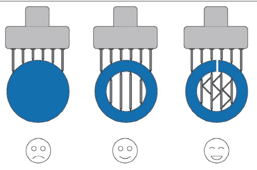
Solid models with large section will lead to printing failure.
