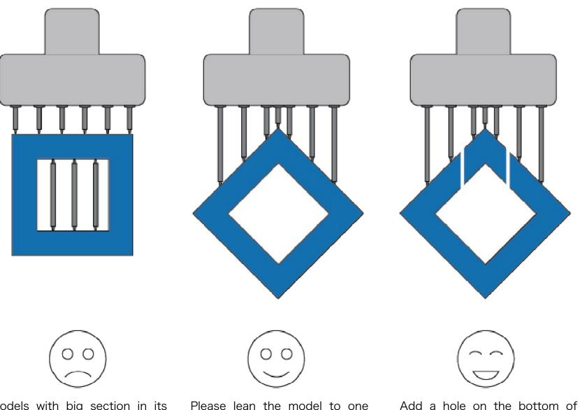
Models with big section in its top and bottom and excessive flat inside need to be added lots of supports. Please lean the model to one direction in some degree to reduce the section, so we can add less supports for the model.
